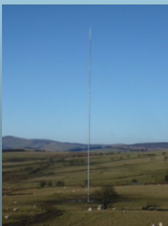
One of the met-masts that a bat detector was attached to for ‘at height’ surveys.
